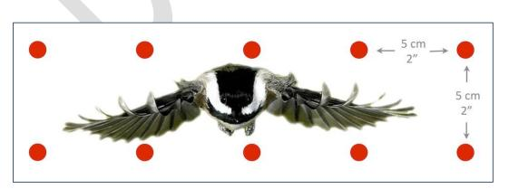
Figure 6: The spacing of markers is representative of the area occupied by a flying songbird, the most numerous victims of collisions (American Bird Conservancy / Safe Wings Ottawa).
